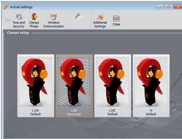
Fig. 33. Reversing the clamp phase.
